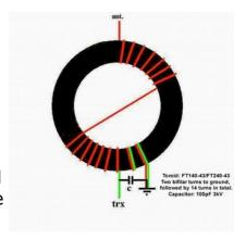
Therefore, 2500 Ohms at the end of the EFHW is transformed down to around
