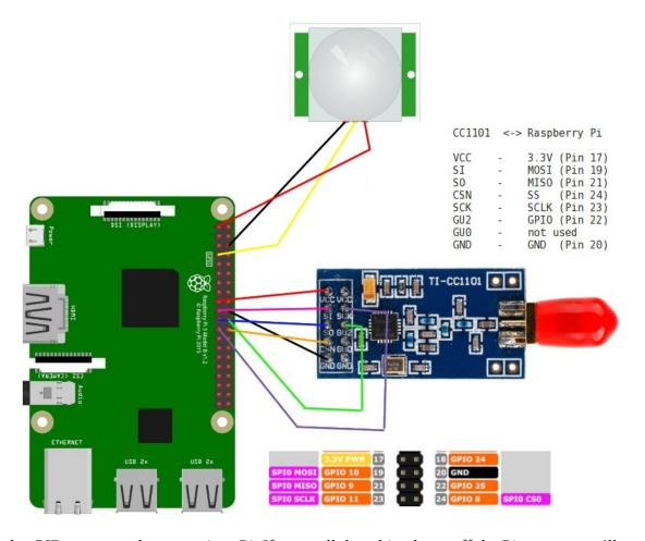
Attach a PIR sensor to the transmitter Pi. If you pull the white dome off the Pir sensor you'll usually see the pin designations screen-printed on the PCB. (radio shown is the old 5x2 pin version)
