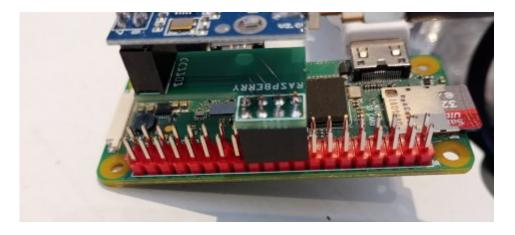
As the adapter communicates over SPI, we need to enable SPI mode on the Raspberry Pi:
