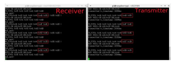
Note: I couldn't get this to work correctly on a Pi5, where the Processor and GPIO pins are abstracted via a microcontroller, and wiringPi support is still quite new (6<sup>th</sup> August 2024) – it locks up after seeming to transmit the first packet. It works fine on Pi4, Pi Zero and even an original Model B running Raspberry Pi OS Lite Bookworm Debian 12.
