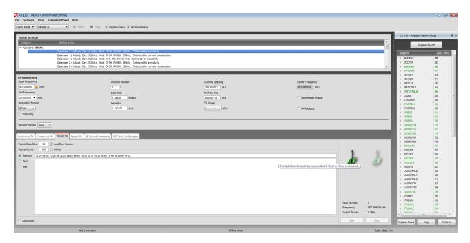
In the center panel you can choose RF Parameters: Base Frequency, Modulation Format, Data Rate and TX Power. When you change these values, the hex values on the right of the screen change too. When all the options are set you can export the Hex values needed to configure the radio by clicking the Register Export button on the top right of the window.
