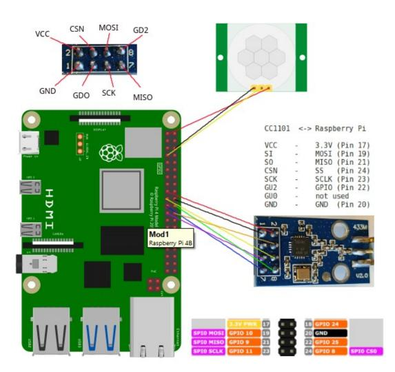
You can attach the CC1101 board to the Pi using regular female to female breadboard cables, or you can use a PCB adapter, like this:
