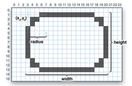
Here's an added bonus trick: because the circle functions are always drawn relative to a center pixel, the resulting circle diameter will always be an odd number of pixels. If an even-sized circle is required (which would place the center point *between* pixels), this can be achieved using one of the rounded rectangle functions: pass an identical width and height that are even values, and a corner radius that's exactly half this value.
