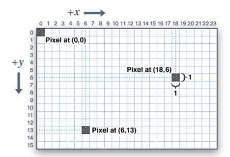
Coordinates are always expressed in pixel units; there is no implicit scale to a real-world measure like millimeters or inches, and the size of a displayed graphic will be a function of that specific display's *dot pitch* or pixel density. If you're aiming for a real-world dimension, you'll need to scale your coordinates to suit. Dot pitch can often be found in the device datasheet, or by measuring the screen width and dividing the number of pixels across by this measurement.
